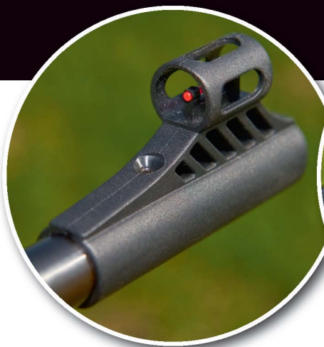
Right and inset: The 280 does feature fibre-optic rear- and fore-sights, with the rear micro-adjustable
